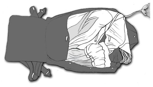
6.4.2 Dressing as you go and keeping the canopy as far outboard and neat as possible, close the right side flap by sliding grommets over Thandles. By keeping the canopy tucked far outboard, you are creating a nest that the pilot chute will eventually snuggle into. Route the bridle out in between the 1st and 2nd grommets of the container.
