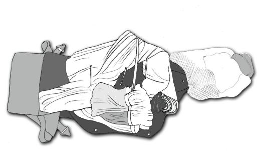
6.3.7 Fold the parachute at the bottom of the container where you extended 5 in past, at a 90° angle towards the center.
