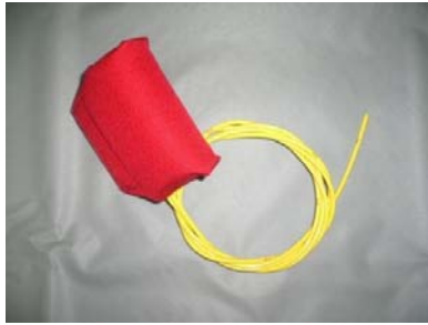
Main cutaway handle with rigid puff
