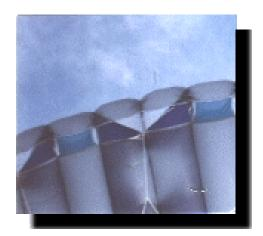
The Icarus EXTreme's cross-braced tri-cells are the key to its ultra-high performance.
