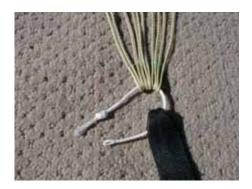
1) Check the continuity of your line group. Begin installation by inserting the link through all the lines and then through the riser.
