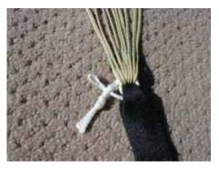
3) Insert the small loop at the top of the link through the loop just above the stopper knot. It may be necessary to use a fid or ballpoint pen to open the loop slightly to allow insertion.
