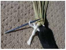
4) Using a fid, ballpoint pen, or similar object, carefully open the top loop a little wider to enable it to pass over the stopper knot. Make sure that you don't damage any of the fibers as you perform this step.
