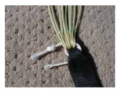
2) Pass the link through the lines and through the riser again, so that the link forms a doubled loop.
