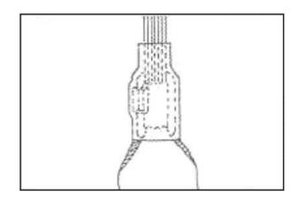
Install the slider with each of the four groups of lines routed through the appropriate slider grommet. When installed correctly, the pull tabs are on the rear of the slider and the slider's reinforcement tape faces up towards the canopy, not down towards the jumper.
