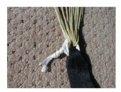
5) Now pass the widened loop over the stopper knot, then "milk" the finger-trapped portion of the link to return the top loop to its original smaller size.
