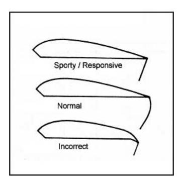
All BLADE canopies are designed to fly correctly for most jumpers with normal brake line length. With this setting it is easy to collapse the slider or pull the front riser, without causing the canopy to buck. The slack in the brake lines at the factory-recommended setting is 10-15 cm. If you find that this toggle setting needs to be adjusted please contact HiPerUSA or your local rigger.
