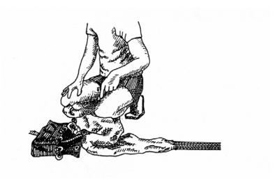
13) Push the canopy into the bag. Make sure that you keep the canopy in a bundle as you go. Push any remaining parts of the canopy neatly into the bag.
