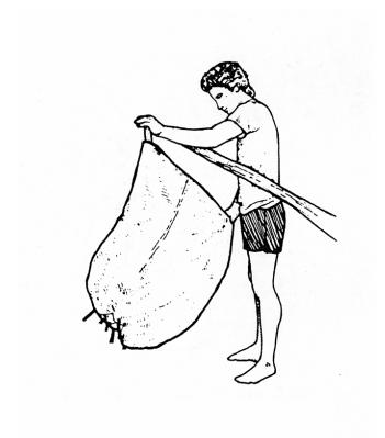
8) Swing the canopy forward, and gently lay it down onto the floor. Take care that the lines remain tight and straight.
