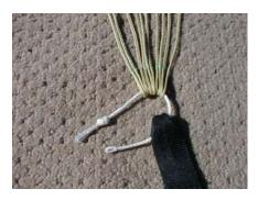
1) Check the continuity of your line group. Begin installation by inserting the link through all the lines and then through the riser.
