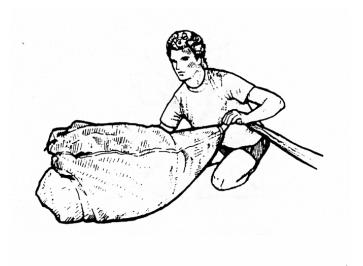
9) Push the lateral canopy parts together and under the bundle. Beginning at the slider, kneel on the canopy and form a "cocoon" the width of the deployment bag.
