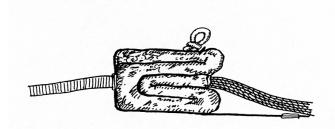
As you stow the suspension lines on the deployment bag, use very small bands and / or make a double-turn of each stow. Because the Technora line is very small, it is important to ensure that the lines release from the bag in proper sequence to prevent hard openings or other deployment problems.
