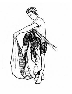
7) Now put the right and left side of the tail around the bundle and roll both sides somewhat together. **Caution:** No control lines should be allowed to pass around the canopy. This could lead to a line-over malfunction!
