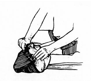
14) If packed correctly, the canopy should lie in the deployment bag as in this illustration.
