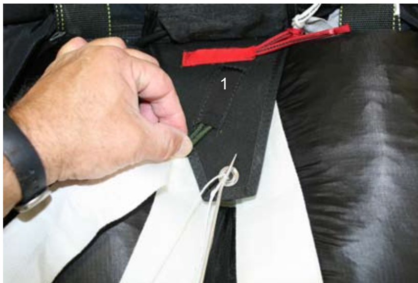
Figure 2-151. Green Loop Installation
