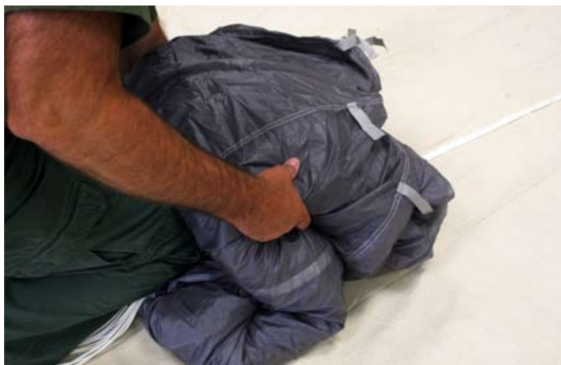
Figure 5-57. Make The Second “S” Fold
