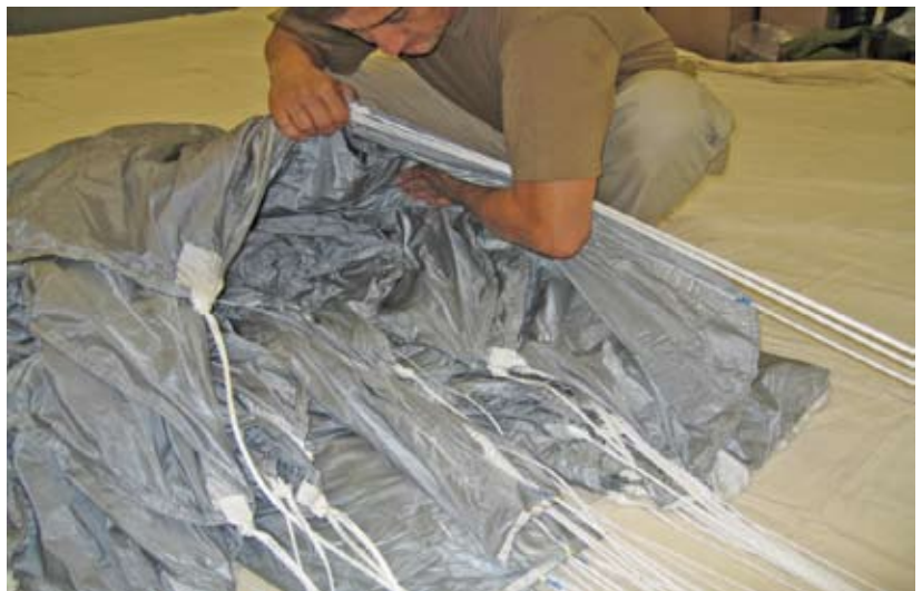
Figure 2-55. Clear Fabric Between Line Groups C & D
