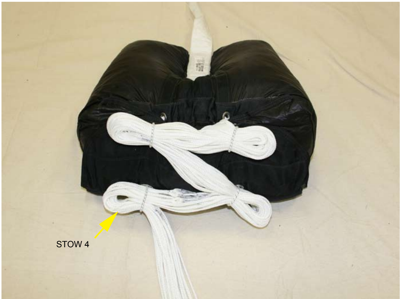
Figure 2-117. Place The Final Safety Stow
