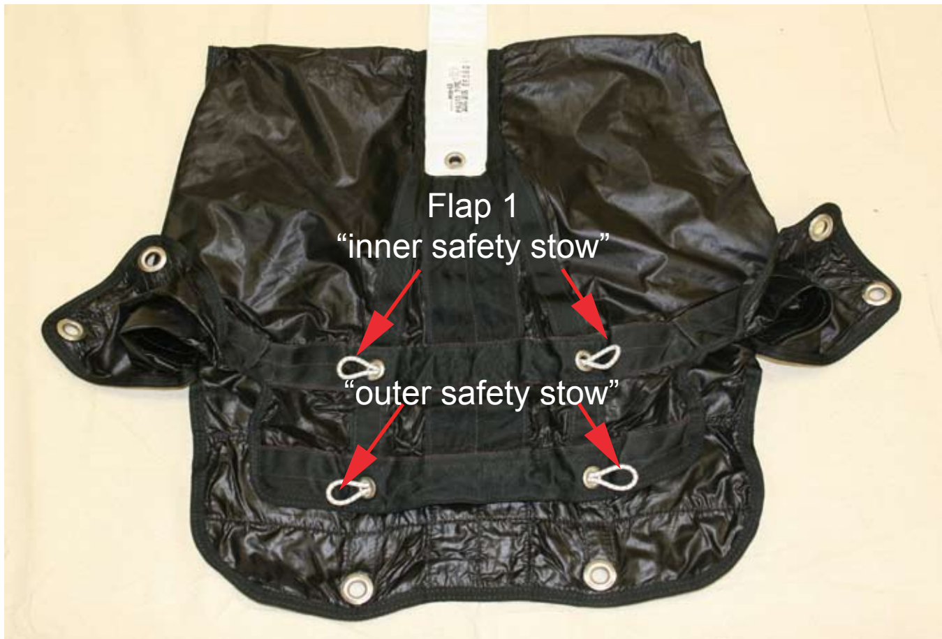
Figure 2-98. Deployment Bag Safety Stow Locations
