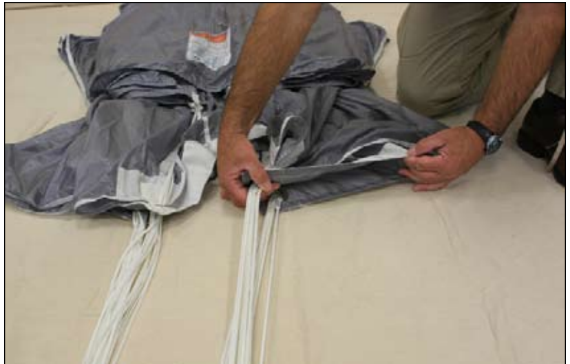
Figure 2-72. Quarter The Slider
