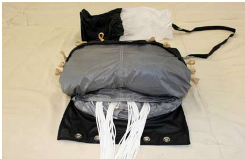
Figure 5-24. Ready For The Locking Stows
