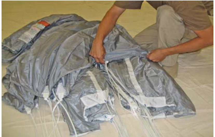
Figure 2-66. Flake The Tail
