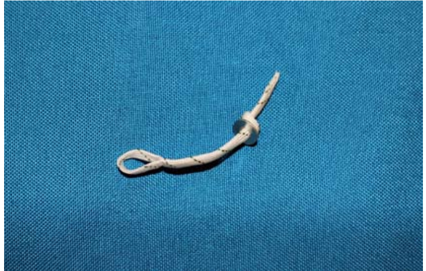
Figure 24. Main Closing Loop
