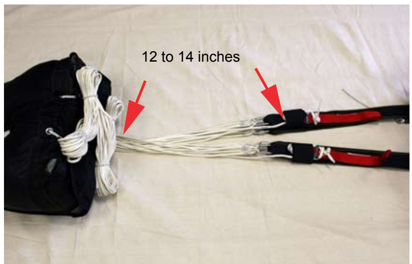
Figure 2-121. Stow Lines With 12 to 14 Inches Remaining
