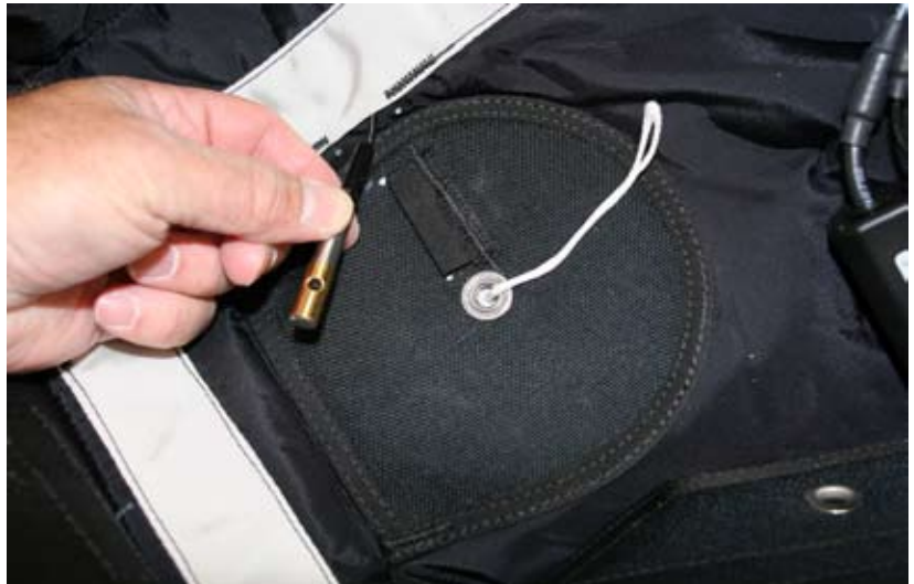
Figure 2- 5. CYPRES Cutter Routing
