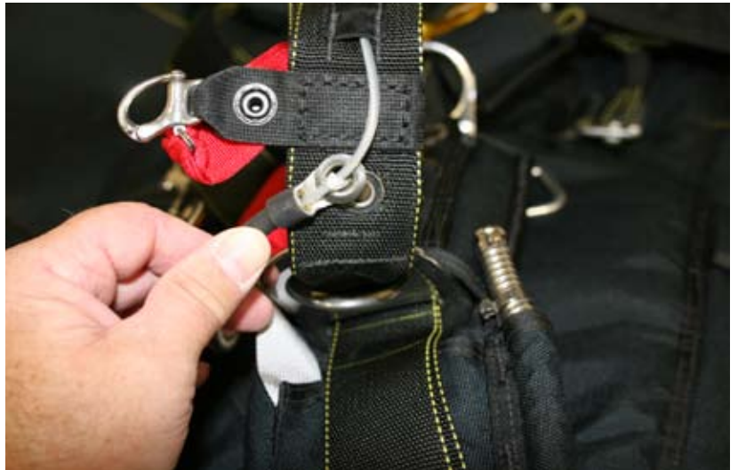
Figure 3-5. Insert The Cable Into The Retention Channel
