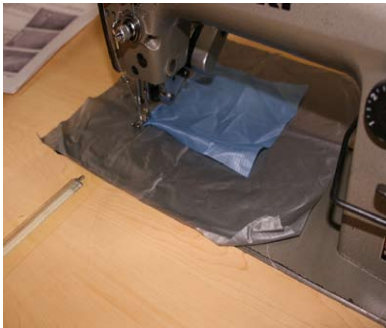
Figure 7-6. First Two Corners Sewn Down
