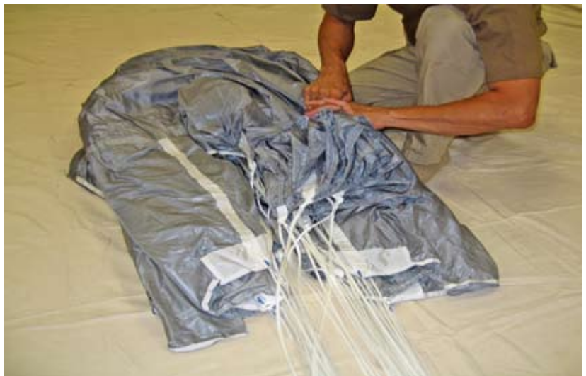
Figure 2-68. Tail Shown Flaked To One Side
