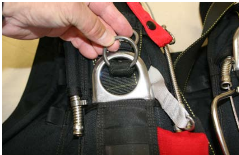
Figure 3-1. Insert Second Ring
