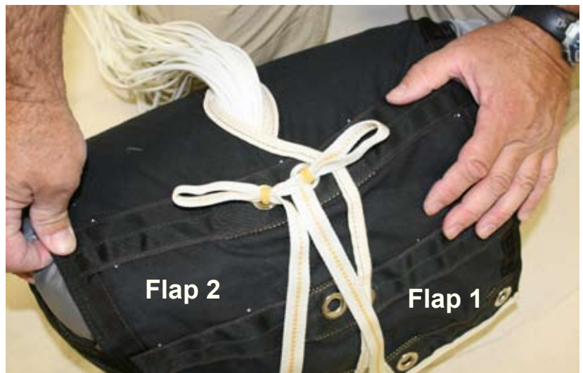
Figure 5-66. Make The Second Bridle Bight
