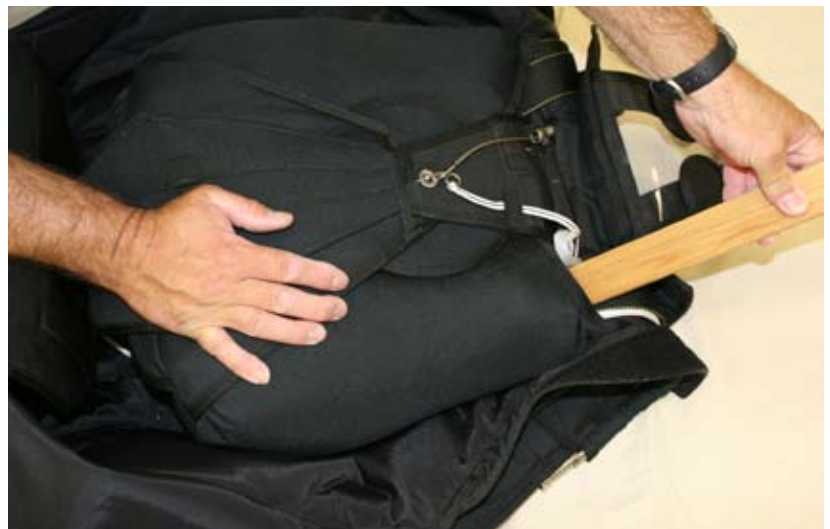
Figure 2-143. Carefully Tuck In The Reserve Tuck Tabs
