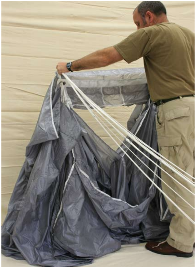
Figure 2-79. Separate The Right And Left Line Groups
