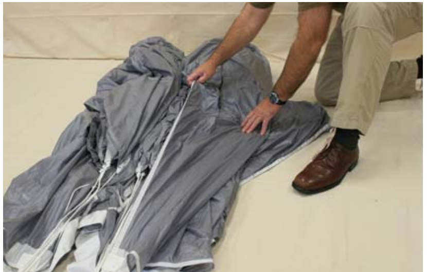
Figure 2-89. Clear The C-D Stabilizers
