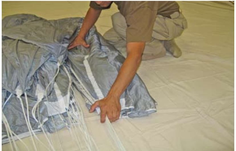
Figure 2-65. Clear The Stabilizer Panel
