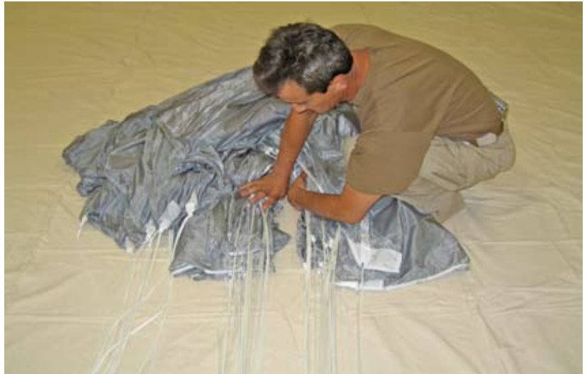
Figure 2-54. Separate The Left & Right Line Groups
