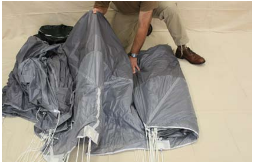
Figure 5.8 Fold The C Line Group Onto The A & B Groups
