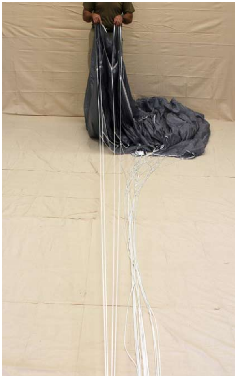
Figure 2-35. Check “A line” Continuity
