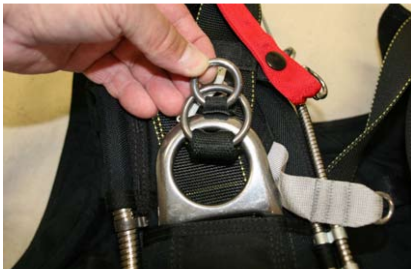
Figure 3-2. Insert Third Ring
