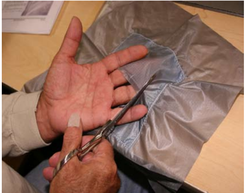
Figure 7-9. Complete Removal Of Damaged Material
