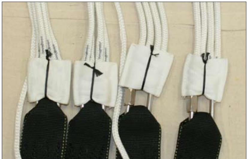
Figure 2-17. Link Protectors Installed
