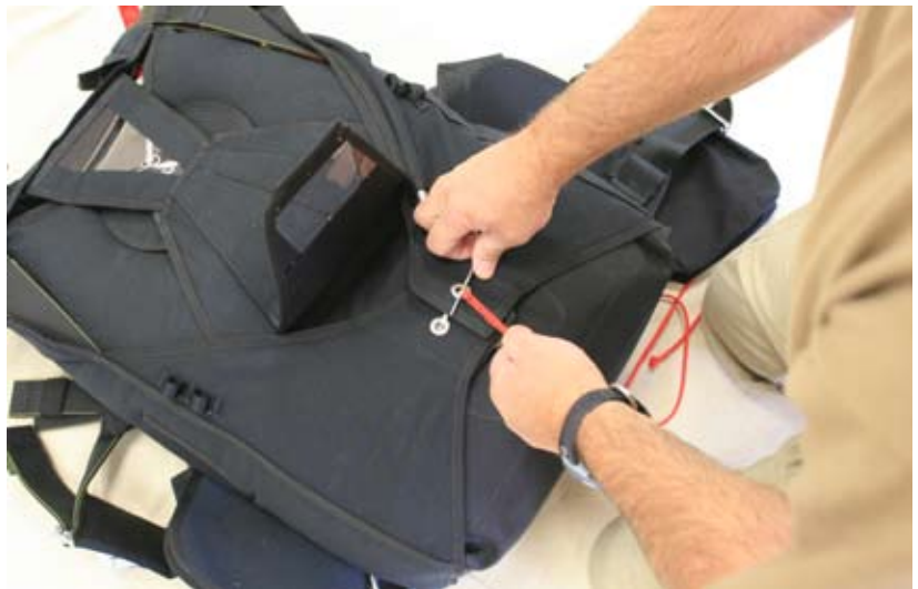
Figure 5-37. Close Flap 4 And Pin
