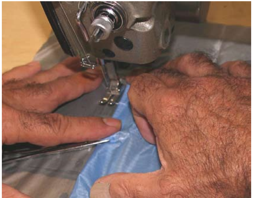
Figure 7-4. Establish The Start Point
