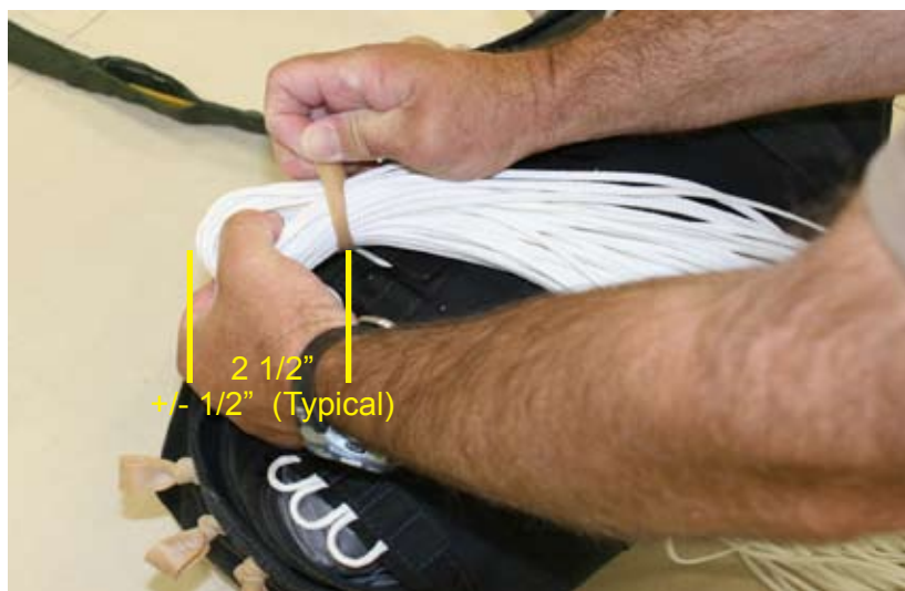
Figure 5-84. Insert First Bight Of Lines
