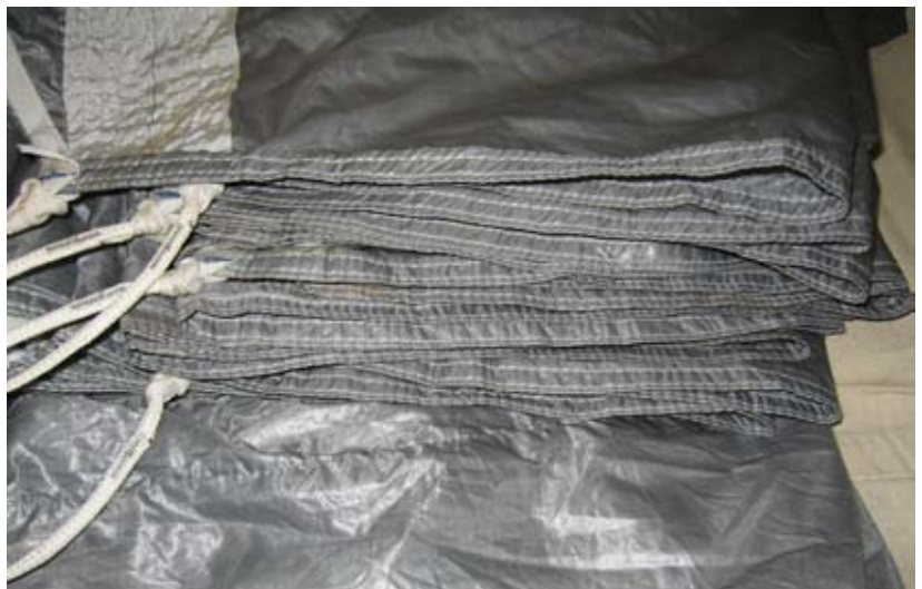
Figure 2-67. Close Up Of The Flaked Trailing Edge
