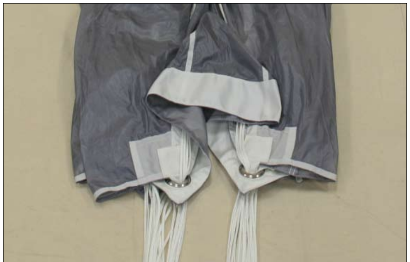
Figure 2-73. Set The Slider
