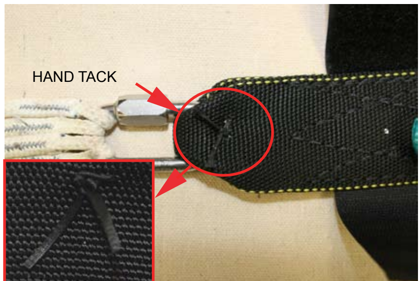
Figure 2-16. Hand Tacked Riser
