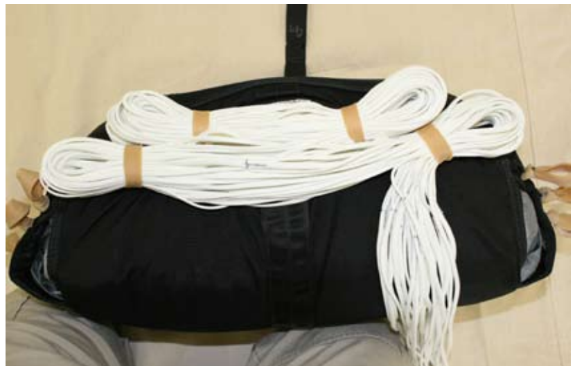
Figure 5-27. Place The Third And Fourth Locking Stow
