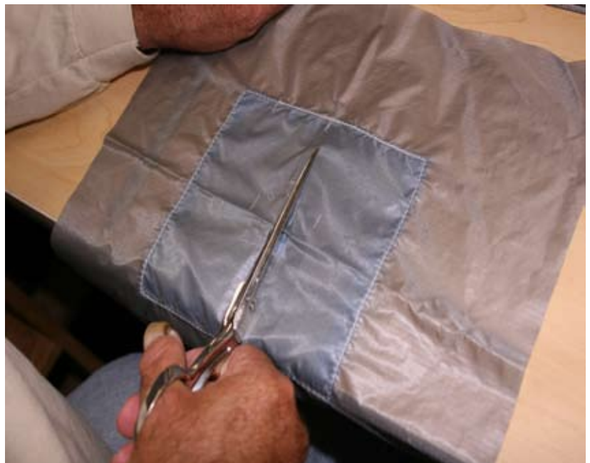
Figure 7-8. Begin Removing Damaged Material
