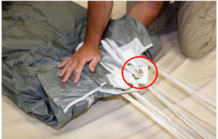
Figure 2-75. Finish The "S" Fold
