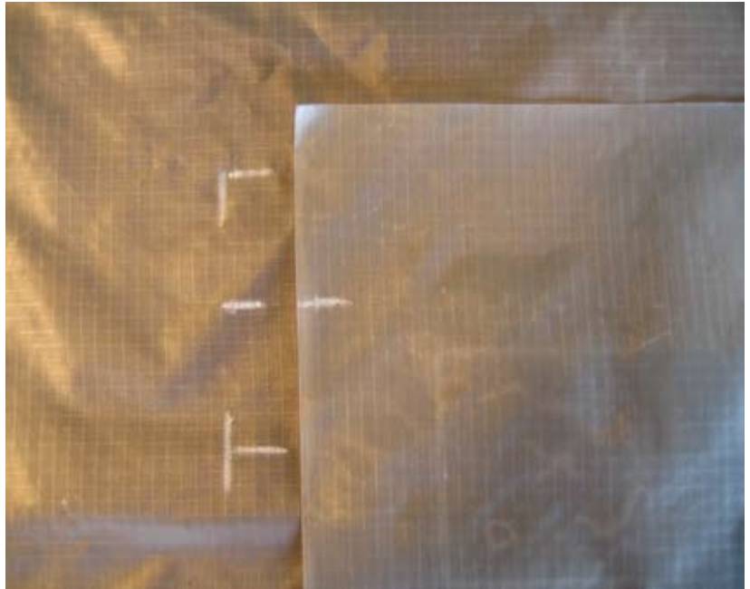
Figure 7-3. Mark The Repair Starting Point
