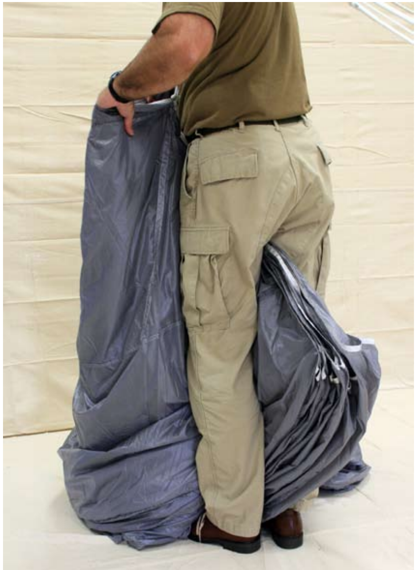
Figure 2-81. Place The Nose Between The Knees
