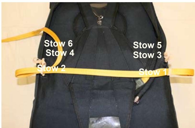
Figure 5-93. Begin To Stow The Static Line
