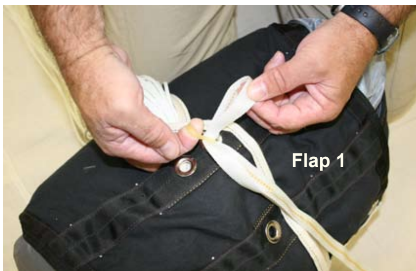
Figure 5-63. Secure First Bridle Bight
